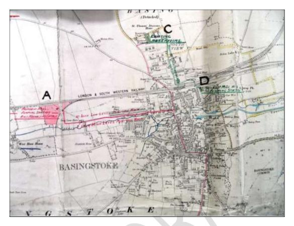
Map 3 *The proposed West Ham pumping station and new pipelines (A), Darlington Road reservoir (C) and existing well and pump (D).*
