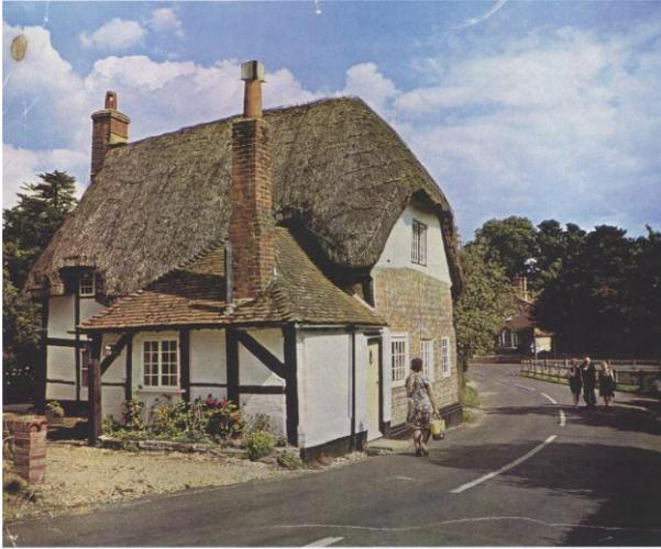
date. The 2-storey house has two rooms with axial spine beams and an end stack and there are many re-used timbers. Both buildings have the small-panel framing and short, straight braces typical of the early 17<sup>th</sup> century and, although they were built
