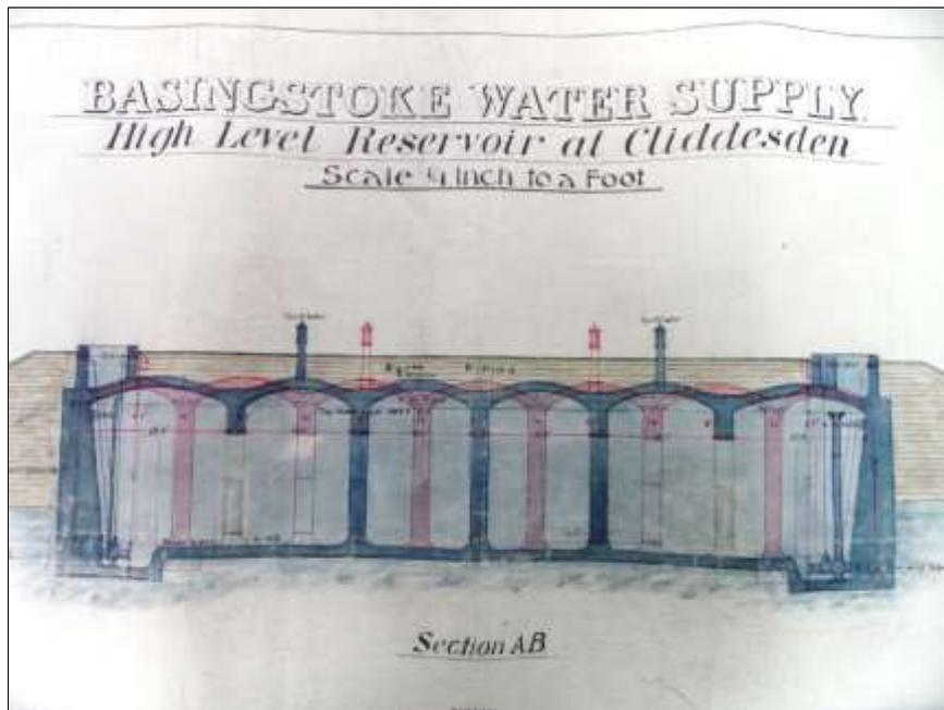
Figure 4 Section through Cliddesden reservoir showing water chambers. The surface outline can still be seen in the landscape (below).
